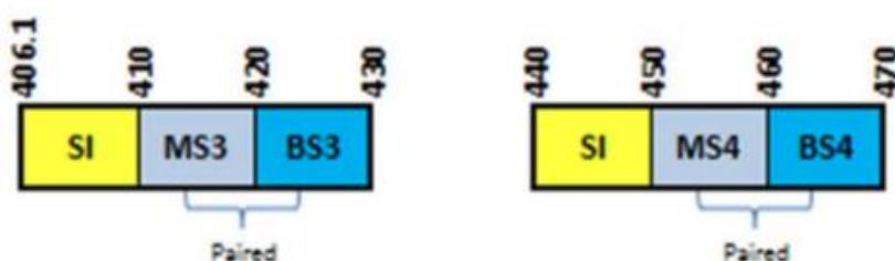
Figure 4.1-1: Illustrative mobile service allocations in the 400 MHz range: Simplex (SI) and paired Mobile station (MS) Base station (BS) use (from [3])
