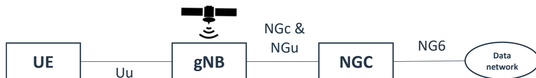
Figure 4.7-2: NTN featuring an access network serving UEs and based on a satellite/aerial with gNB on board
